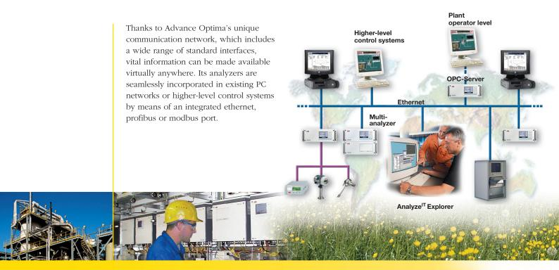
Improved operating functions such as remote control of the analyzer, effective asset management as well as the installation of new software versions from a central maintenance computer, are now also possible. And advanced software tools are available too. Naturally, today's commonly used fieldbus systems are supported by the system as well as the traditional 4...20 mA analog outputs.
